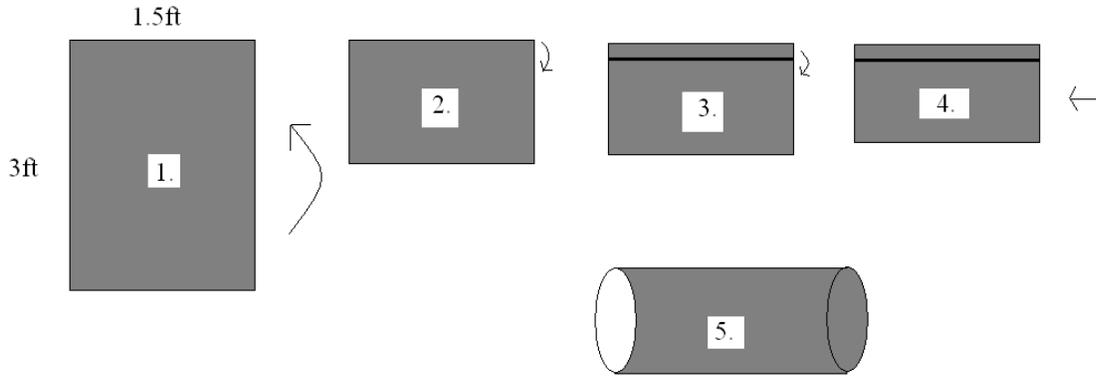
**Figure 2.** How to form the cylindrical section of the funnel traps.
