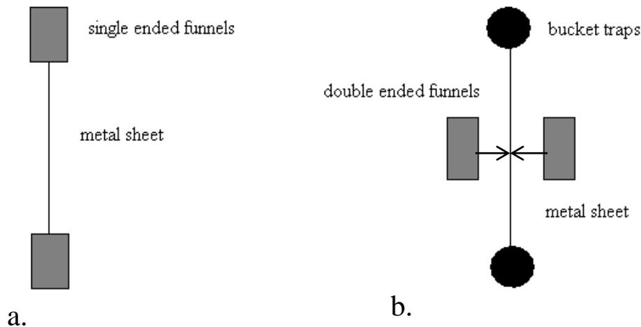
**Figure 6 a,b.** (a) *Drift fence trap array setup at the upland pine and old field sites.* (b) *Drift fence trap array setup at the hammock site.*
