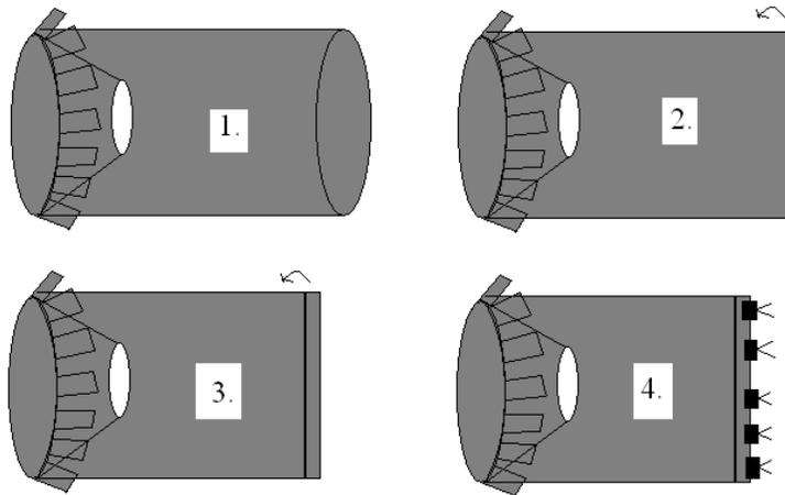
**Figure 5.** *How to form the closed ends of the traps with single funnel ends.*
