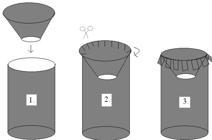
**Figure 4.** *How to attach the funnels to the cylindrical section of the trap.*
