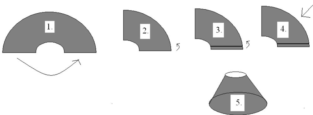
**Figure 3.** How to form the funnels for the traps.
