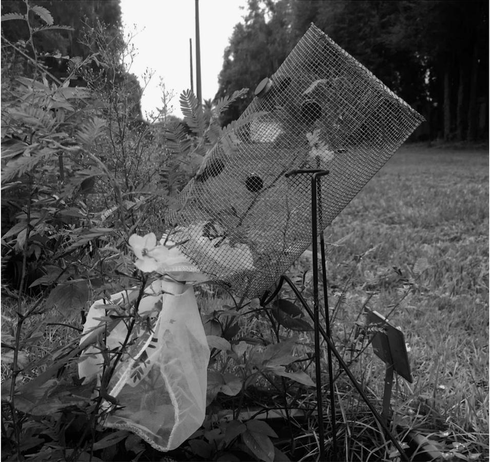
FIG. 1.—An example of a cylindrical small cage (35.6 cm length and 20.3 cm diameter) containing a partridge pea stem that was used for this study. A nylon mesh was affixed to the bottom of the mesh cage so that plant stems could be enclosed within cages without breaking them. Small black circles on the pictured cage are magnets holding a panel. The panel could be removed and mature seed pods gathered without having to take the entire stem out of cage
