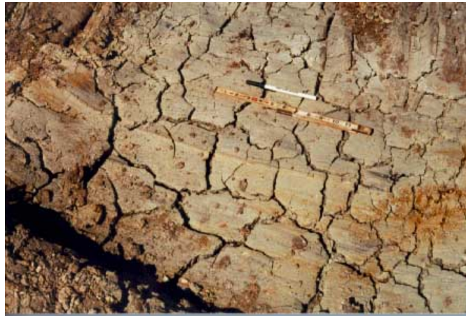
Fig. 3. Clays crack when dry and swell when wet.
